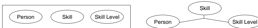
Fig. 1. Two equivalent notations of the ternary SCM association (Person, Skill, Skill Level)
